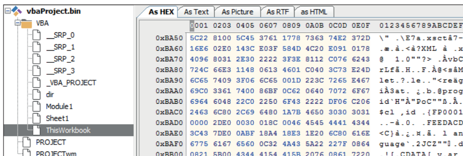
Figure 25: Macro storage in the ‘ThisWorkbook’ stream of an OOXML file.
