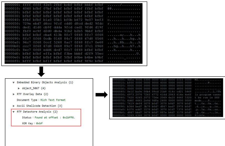
Figure 5: The SAE extracts the data consumed by the 'datastore' control word and then passes it to the stream analyser.
