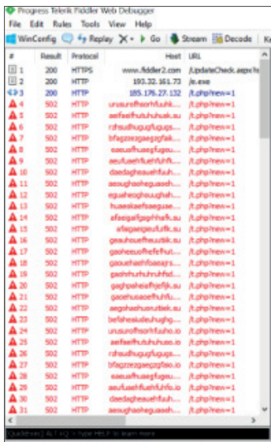
Figure 6: Most HTTP queries result in 502 errors.
